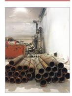
The Comacchio MC 8 D performing auger drilling and the drill pipes
