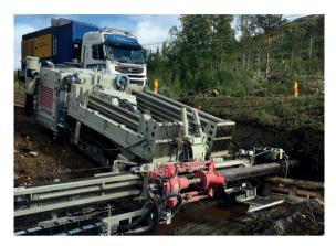
independently via Comacchio's proprietary radio control system that allows controlling all machine functions, from tramming to set-up and drilling.
