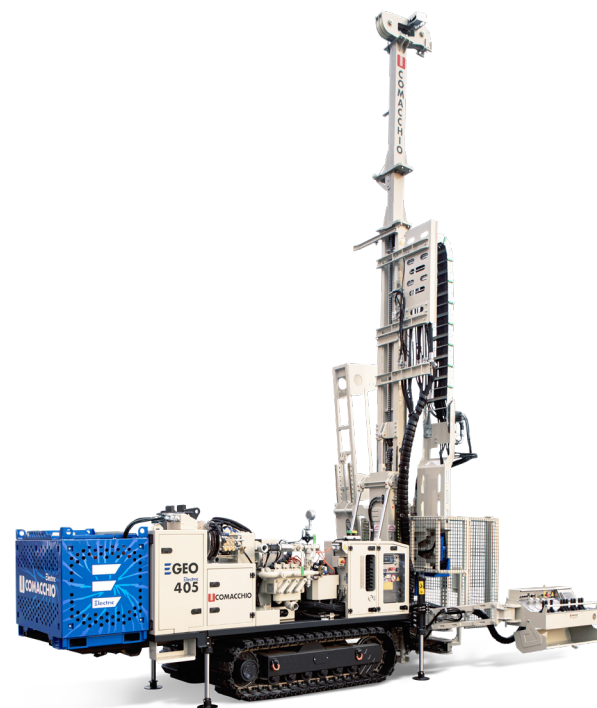
↑ The battery system powering the eGEO 405 is placed on the rear part of the machine in a separate box designed to be easily exchangeable using a forklift or telehandler
