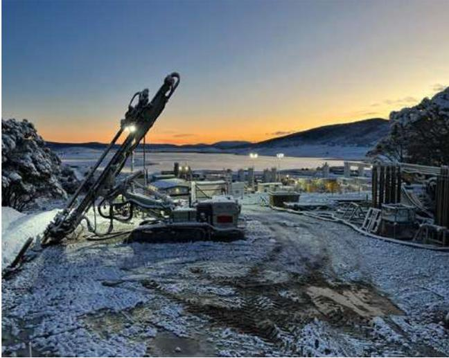
*Grouting work carried out with the aid of a Comacchio MC 22 rig allowed tunnelling to continue on the Snowy 2.0 project after a sink hole developed stopping the TBM*
