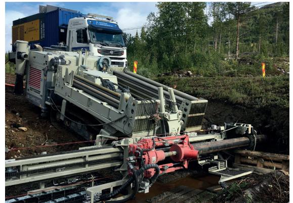
independently via Comacchio's proprietary radio control system that allows controlling all machine functions, from tramping to set-up and drilling.
