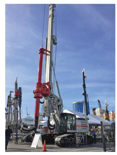
Presented during CONEXPO-CON/AGG 2017 in Las Vegas, the CH 650 is the latest addition to the Comacchio line-up of piling rigs. The launch of this machine follows the introduction in late 2015 of the CH 450, the first machine designed by the Italian manufacturer for the large diameter market.
