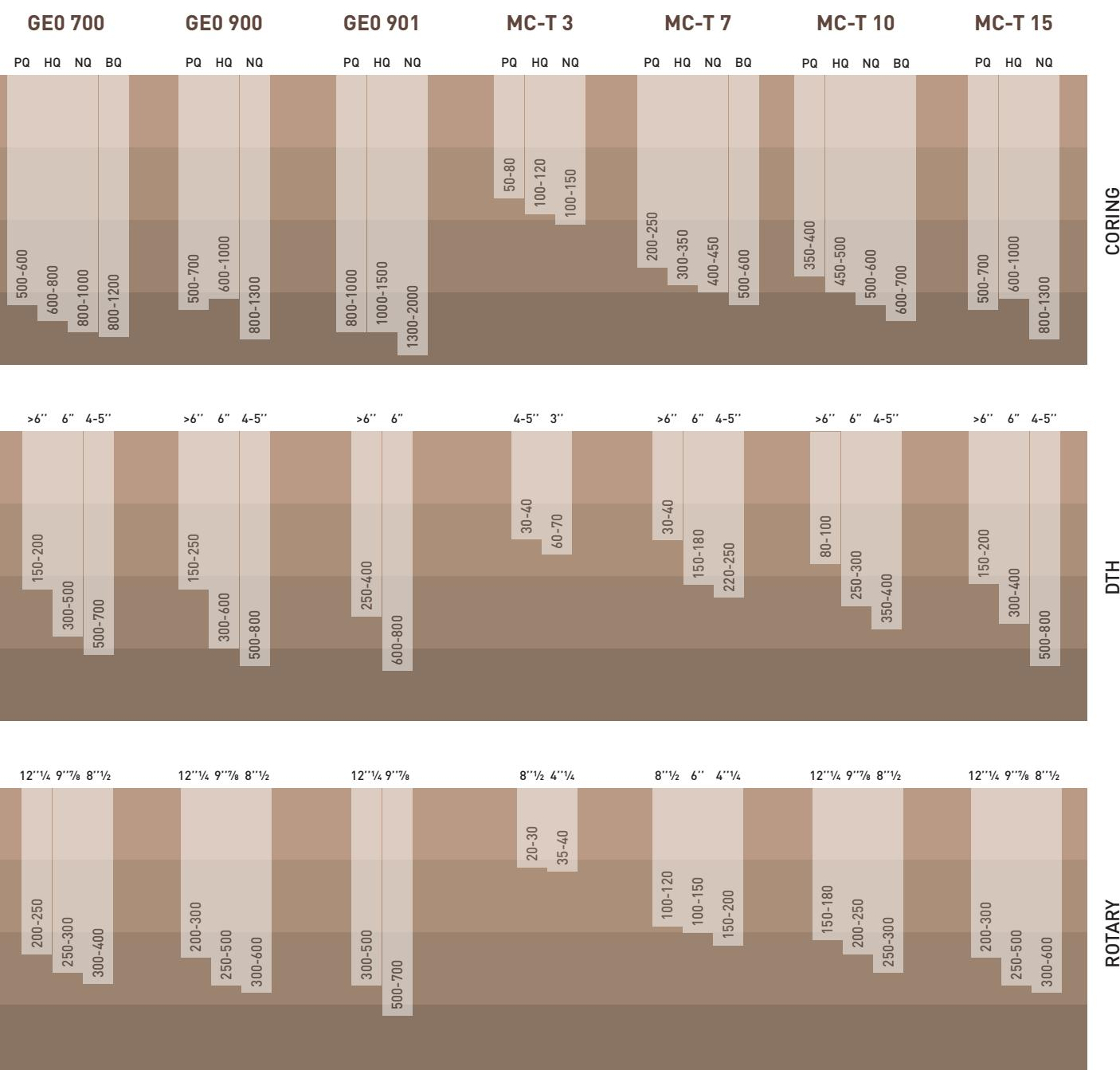
The above data are for guideline purposes only and are calculated for 90° holes, they are subject to: soil conditions, drilling tools, flushing method and other parameters that influence the drilling.
